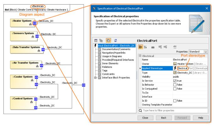
Matching the diagram aspect *Electrical* with the port stereotype name *Electrical*.
