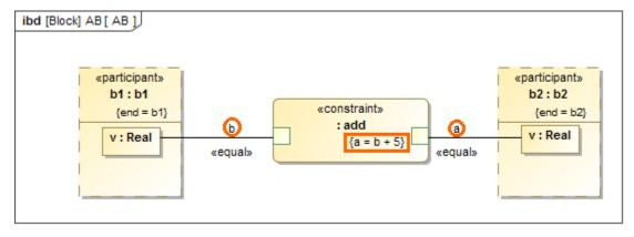
An Association Block can provide or add anything such as Behaviors and connectors (a, b) so signals can flow. Parametric and all other constraints (a = b + 5) work automatically.
