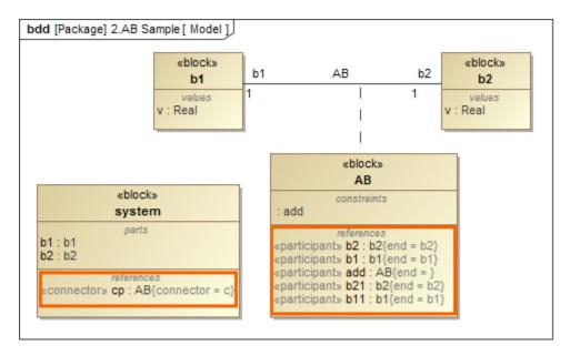
System initializes «ConnectorProperty» by an Association Block instance according to "Connector" reference (AB) and «ParticipantProperty» (b2, b1. add. b21. b11) according to "End" reference (b1, b2).
