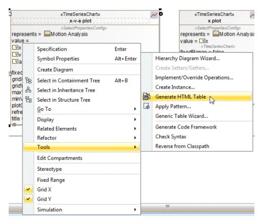
2. This will generate an HTML file, which can be viewed either online or offline. A message stating, "INFO: HTML table(s) is/are generated to the C: \Users\Downloads\CoffeeMachine\_test1 folder, " in the Console pane will appear in the **Simulation Console** pane.
