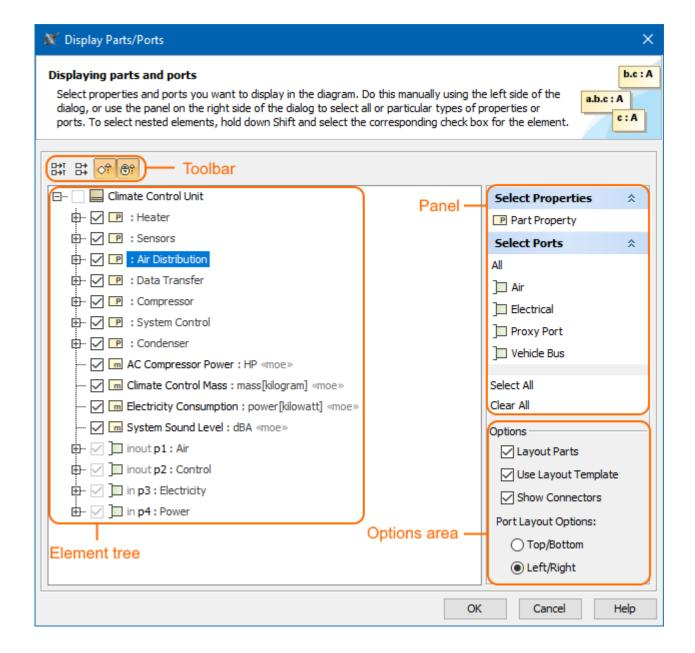
The following procedure will guide in working with the **Display Parts/Ports** dialog when you want to display required ports and properties on the diagram pane.
