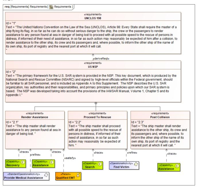
An example of requirements diagram created using the SysML standard
