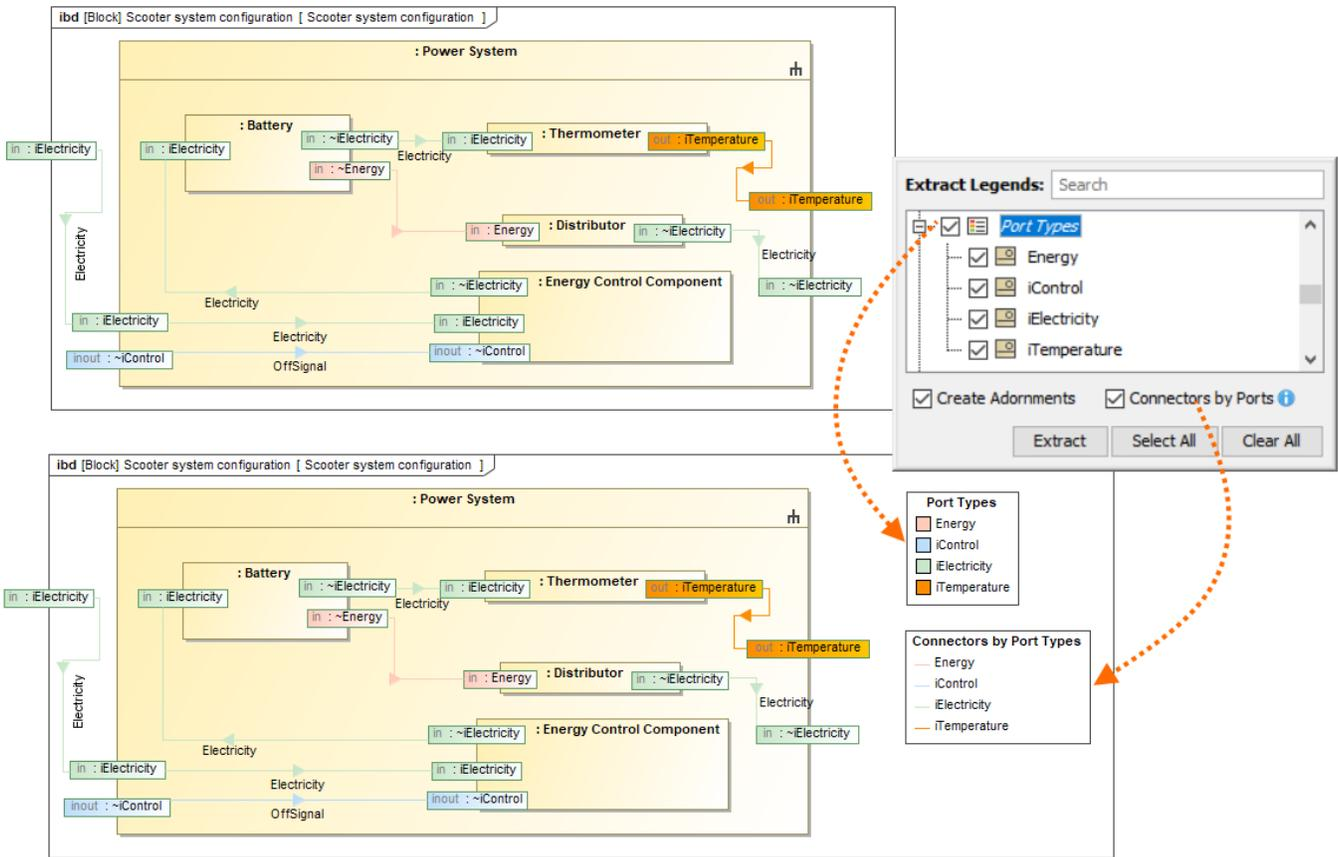
Extracting the Port Types legend according to the elements displayed on the diagram as symbols.
