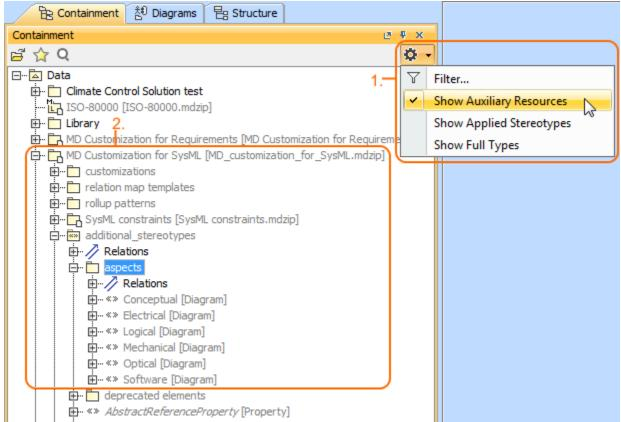
The location of the predefined diagram aspects in the project when SysML plugin is installed. The illustration displays concepts from SysML Plugin.
