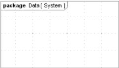
When a new diagram is created, the diagram stereotype icon is displayed on the diagram frame header by default, though you can change it to the context stereotype icon.
