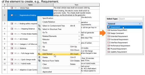
Select the specific table element to nest an additional element within, click the Add Nested button in the table toolbar, and specify the type of the
