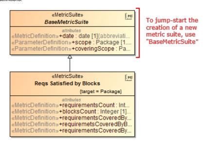
Once the metric suite is created, you can calculate the metrics for a selected element. Analyze the results of the calculations, that is, metrics, in a metric table, which is automatically created for these metrics representation. You can easily reorganize the columns of the table, calculate new metrics, and recalculate the existing metrics with other parameters.
