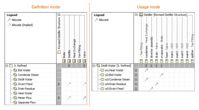
The definition and usage modes in the SysML Allocation matrices.
