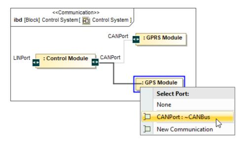
The Select Port menu opens after drawing the Connector from the CANPort Port to Part Property typed by GPS Module Block.
