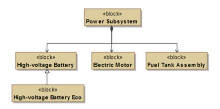
The figure above displays composition and inheritance structure between blocks. If a composite block depends on a particular element, the whole block also depends on this element. The same situation exists with inheritance between blocks. Inherited elements indirectly depend on the elements to which the parent element has relations. These indirect relations are referred to as implied relations, and can be displayed in a dependency matrix, as shown in the figure below.
