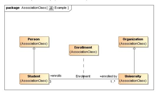
The above example shows the "Enrollment" UML Association Class, which as an equivalent, shorthand meaning to the next diagram. Note that the expansion of the "Role" concepts will be explained here. Similarly, the Facet Of stereotype will be explained here.
