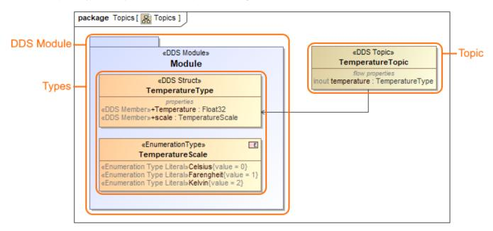
The example of the DDS Topic Definition Diagram where main elements are highlighed: DDS Module, Types and Topic.
