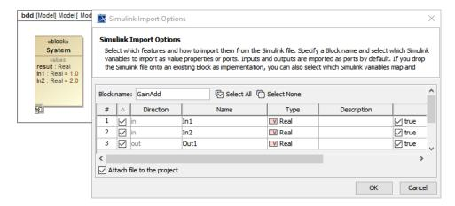
The Simulink Import Options dialog is shown after dragging a Simulink model into the Block Definition diagram or Internal Block diagram of the project.
