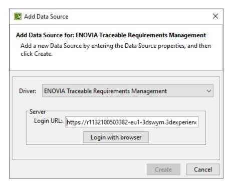
The Add Data Source dialog enables the connection to TRM by entering the 3DEXPERIENCE address for the login.
