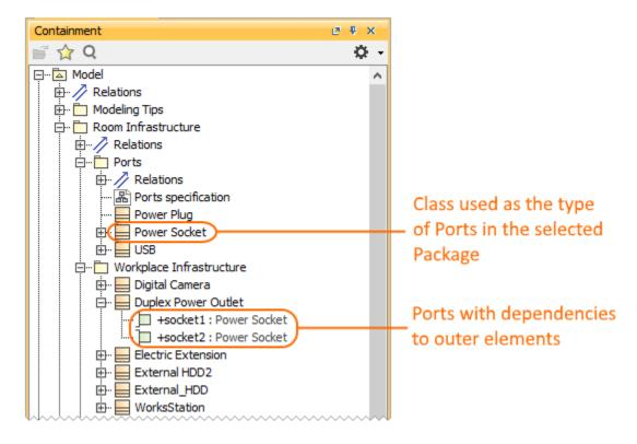
The content tree of a sample model with the Workplace Infrastructure Package having dependencies to the outer elements of the model.
