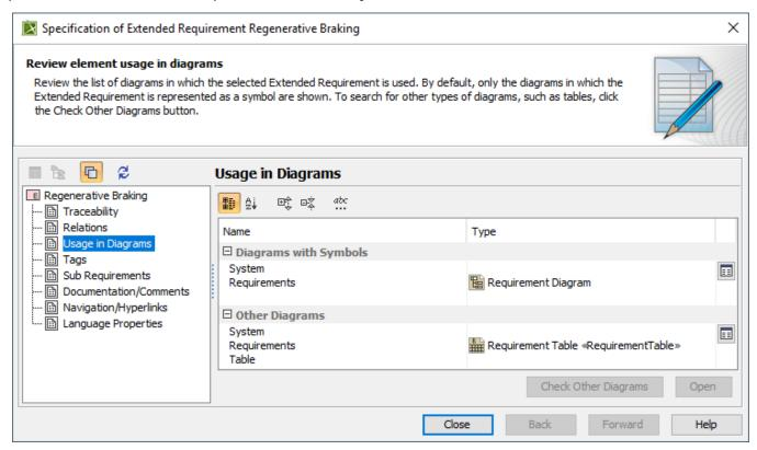
The Specification window of a model element displaying all the diagrams it is used in.
