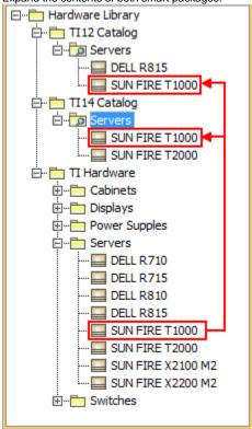
the block SUN FIRE T1000 appears in both TI12 Catalog and TI14 Catalog, since it has both tag values Used In=TI12 and Used In=TI14.
