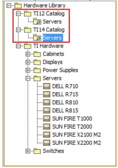
3. Define criteria for gathering the contents of the smart package Servers in T112 Catalog. Specify search options to find in the package TI Hardware, all block type elements with tag value Used In=T112.
