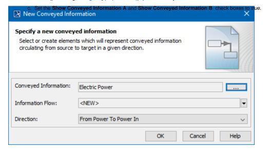
🖺 new Information Flow is set on a Connector that is represented in other diagrams, the new Conveyed Information is displayed only on the diagram on which you set it. You can reverse the direction of the Information Flow on Connectors. How to reverse direction >>
