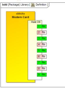
The comparison of default and defined appearance of the Modem Card Block, style, and the position of its ports. The illustration displays concepts from SysML Plugin.
