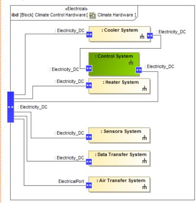
Usage of a layout template with aspect. The illustration displays concepts from SysML Plugin.
