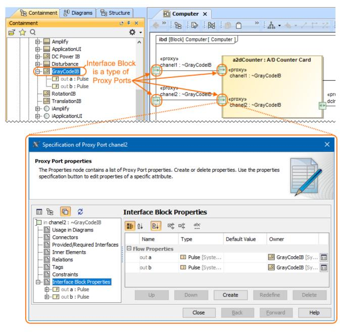
The GrayCodelB Interface Block is a type of Proxy Ports.
