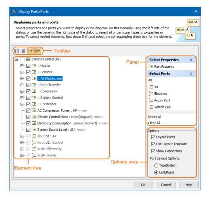
The following procedure will guide you in working with the **Display Parts/Ports** dialog when you want to display required ports and properties on the diagram pane.
