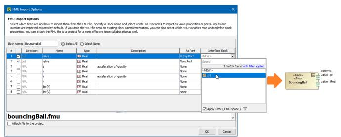
Selecting the Proxy Port and an Interface Block upon the external model import.
