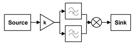
This example portrays the signal flows between system components. The signal flow is unidirectional, and physical conservation laws do not apply in these applications because the same signal can be sent to multiple receiving components. In this model, the function generator is being amplified and then sent to parallel filters (one high-pass filter and one low-pass filter), until the mixer combines the filtered signals for the final signal processor output.
