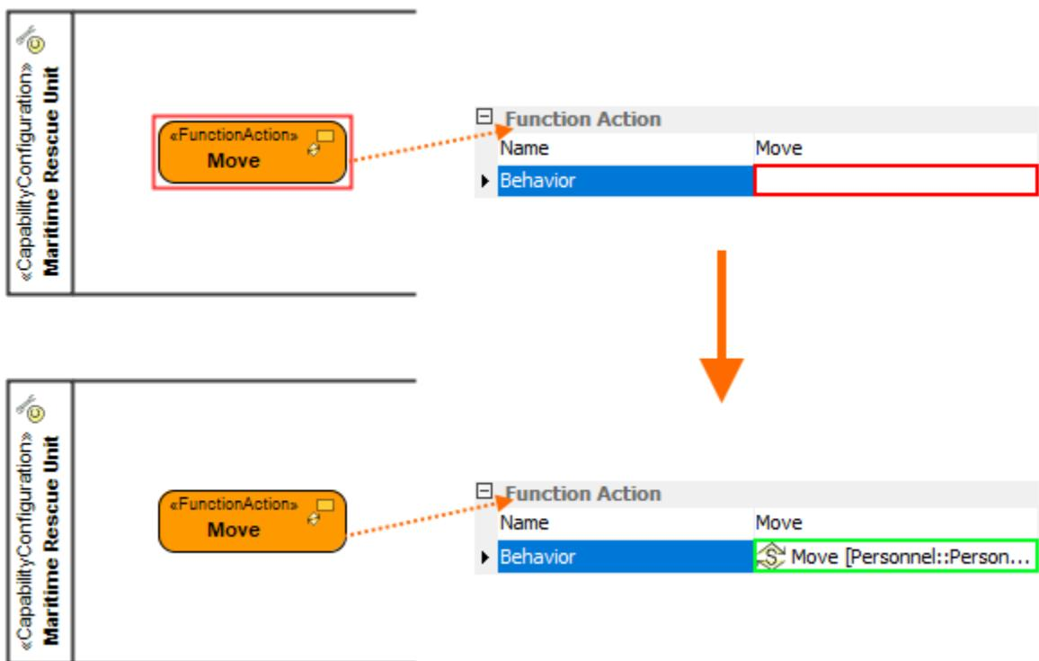
Behavior of Function Action is specified using Select Behavior solver
