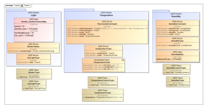
The example defines three packages or DDS Modules for the three factor that we would like to measure and control.
