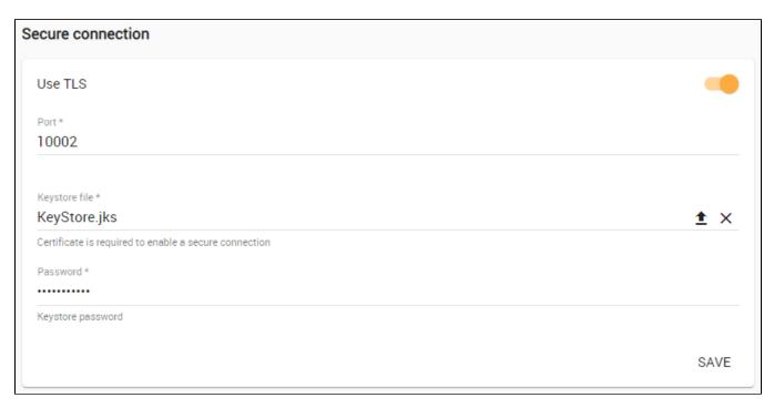
Enabling TLS protocol in TWCloud (when the option is turned on, the color changes to orange).
