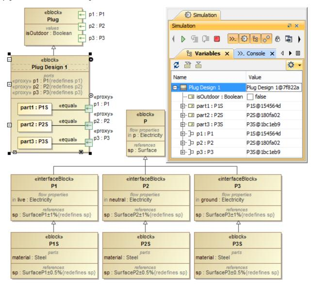
The target Objects of proxy Ports are visible when the Ports connected by Delegation Connector.
