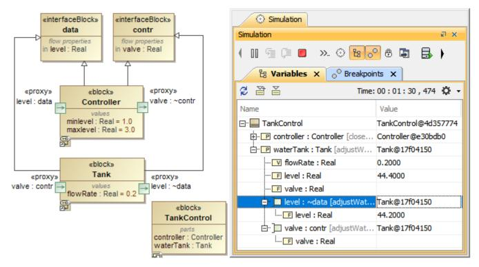
Proxy Port nodes (level and valve) show only features defined by «interfaceBlock» (level and valve Flow properties).
