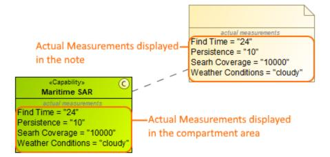
To display measurement values in the compartment area of the element shape
