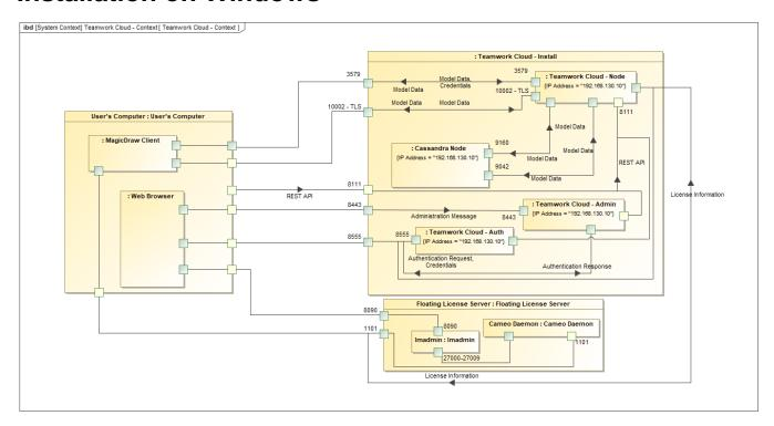
This section provides instructions on how to install Cassandra and Teamwork Cloud on Windows. During the installation, the installer asks you to provide the required configuration values and creates a Windows service for you.
