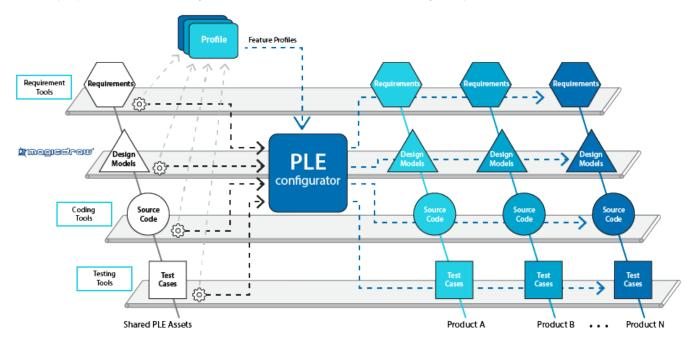
MagicDraw dynamically creates a system model of a particular variant
