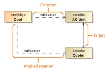
In the example above, the value of the **Target** parameter is a generalization (direction – **Target To Source**). This means that starting from the *AC Unit* block, all composed blocks are collected. In this case, the *Cooler* block is the result of the **Target** parameter. By default, the values of the **Target** parameter are simple navigation operations - a generalization (direction - **Target To Source**) and part (direction - **Target To Source**).
