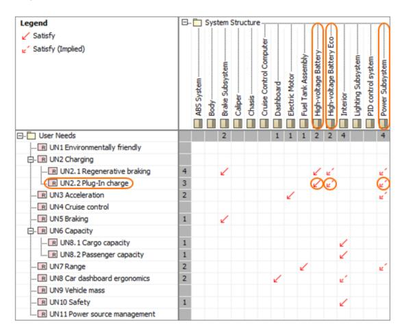
As shown in the figure, the *High-voltage Battery* block satisfies the *Plug-in charge* requirement. According to the composition and generalization, the *Power SubSystem* and *High-voltage Battery Eco* blocks should satisfy this requirement as well. In the matrix, these relationships are shown as implied, and marked with red, dashed arrows.
