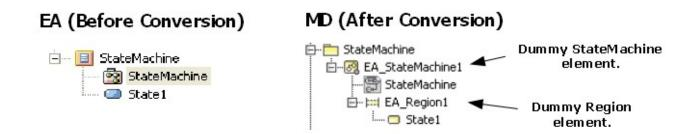
A dummy StateMachine element and a dummy Region element.
