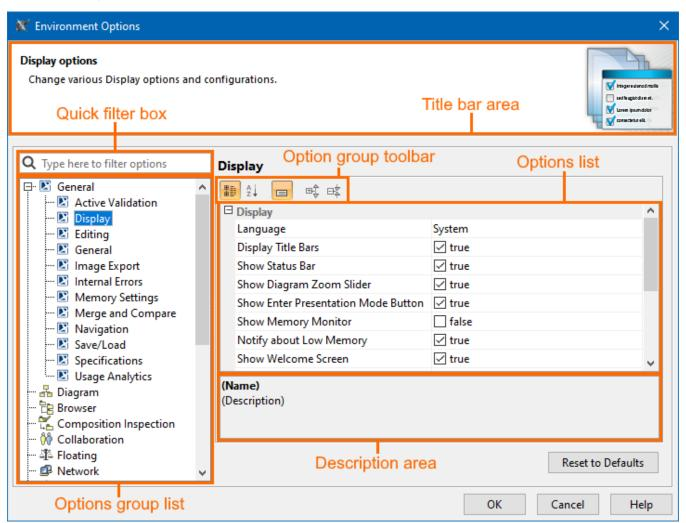
The **Environment Options** dialog contains various project-independent options grouped by different features (for example, diagrams, Model Browser, code engineering). Each option group is available in a different tab. Tabs are displayed in the tab tree.
