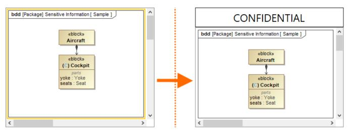
The diagram contains an element symbol with an added Data Marking (C) but the Diagram Banner is not created for the diagram. The error is resolved by creating the Diagram Banner via the **Create** solver.
