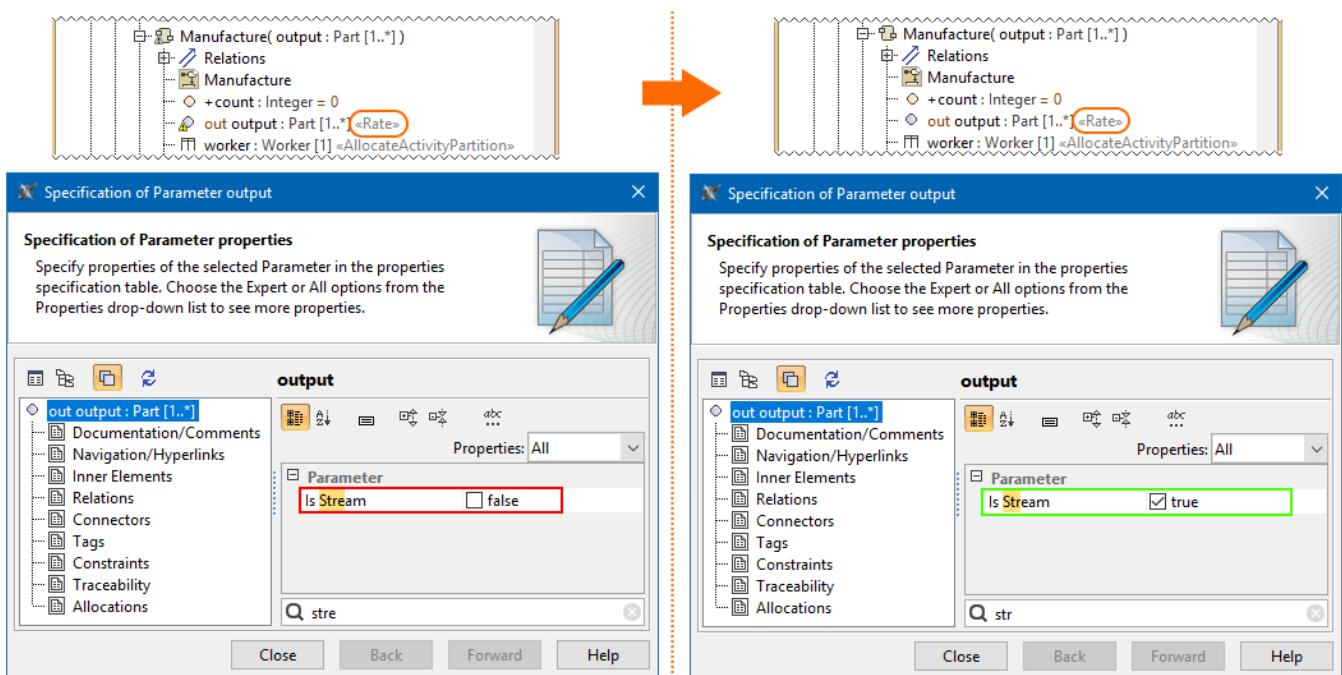
The output Parameter must be streaming if it is stereotyped by «rate».
