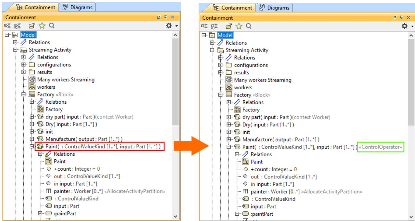
The *out* Parameter type is ControlValueKind enumeration and its *Paint* Activity must be stereotyped by «ControlOperator».
