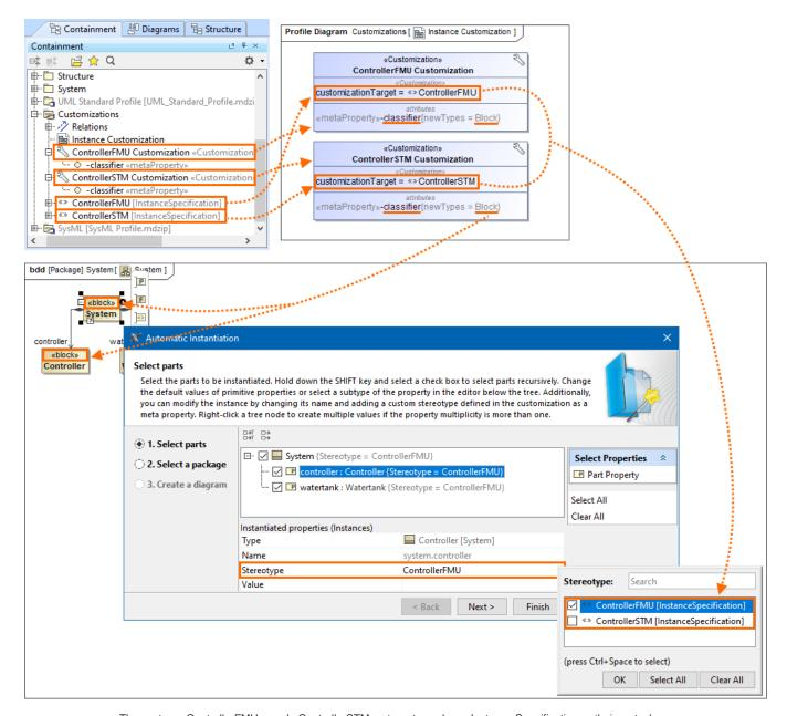
The custom «ControllerFMU» and «ControllerSTM» stereotypes have *Instance Specification* as their metaclass and their respective customizations *ControllerFMU Customization* and *ControllerSTM Customization* have a meta property named classifier with the **New Types** property value set to the «Block» stereotype.
