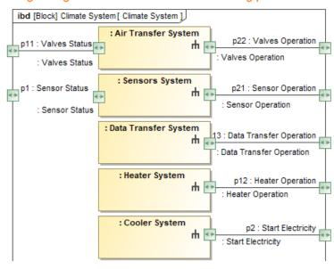
The selected Part Properties in the Climate Control IBD are extracted. As a result the new climate System Block and the SysML Internal Block Diagram are created.
