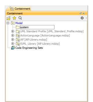
Click on the system package and create a new Class diagram in the package by clicking the Cre ate Diagram button on the toolbar. The Create Diagram dialog will open (see the following figure). Select Class Diagram.
