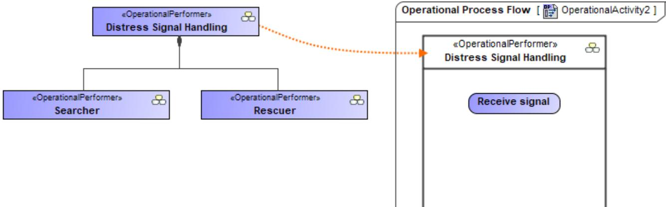
The Operational Process Flow diagram is created. In the Swimlane, you can add either Operational Activity Action or Operational Action. In both cases, you can create an inner Operational Process Flow diagram for an Operational Activity Action or Operational Action Smart Manipulator toolbar.
