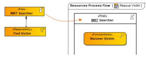
The Resource Process Flow diagram is created. In the Swimlane, you can add either Function Action or Resource Action. In both cases, you can create an inner Resource Process Flow diagram for a Function Action or Resource Action Smart Manipulator toolbar.
