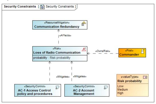
An example of the Security Constraints diagram
