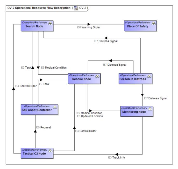
The Operational Connector established in an OV-2 can be realized by resources and their interactions in a SV-1 Systems Interface Description model or Sv cV-1 Services Context Description model.
