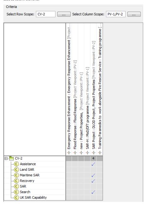
This model is analogous to the SV-5a Operational Activity to System Function Traceability Matrix, but provides the interface between Capability and Actual Project models rather than Operational to System Models.
