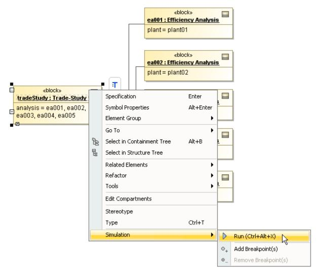
You can run an Instance Specification whose Classifier is a Behavior. In such case, Cameo Simulation Toolkit will initialize the object from the Behavior and load the slot values to the object. Then it will simulate the object in the same way as it simulates the object initialized from a Behavior.
